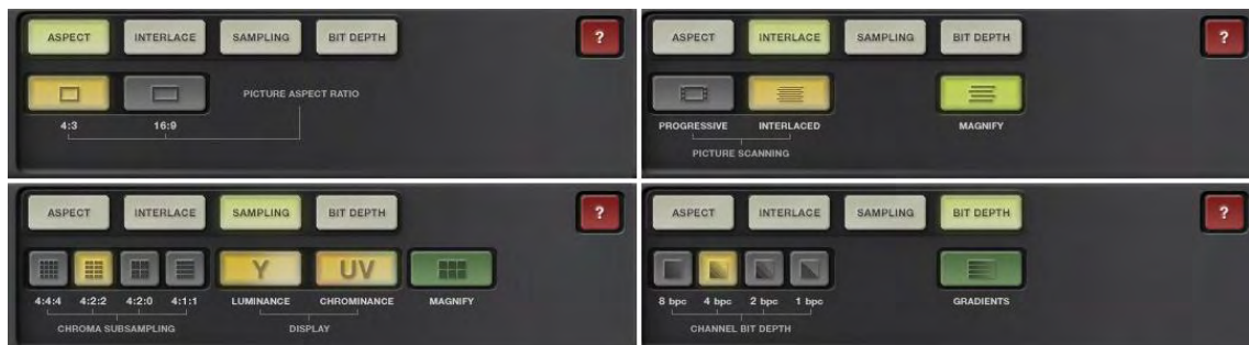
Figure 2. VideoLab’s four simulations modes – Aspect Ratio (top left), Interlacing (top right), Luminance, Chrominance and Sampling (bottom left), Bit Depth (bottom right).
