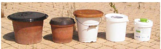
Figure 3. Project "fridge in a vessel": Comparing the cooling by means of evaporation of water in different vessel
