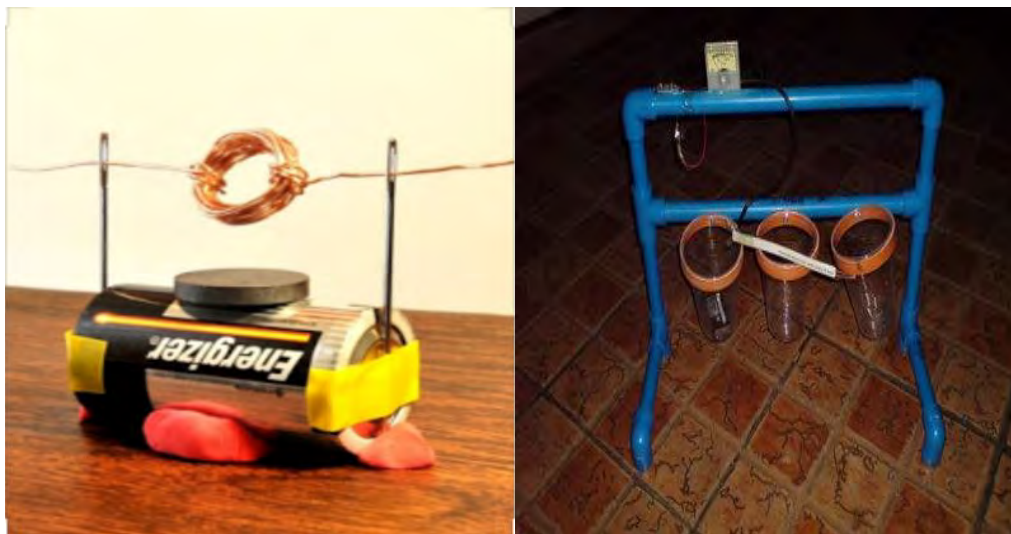
Figure 2. Improvised resources designed to explain the operation of a direct current motor.
