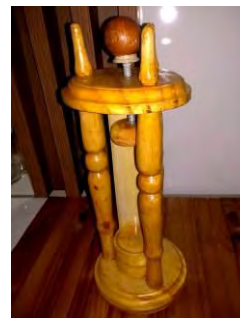
Figure 3. Third pile built: the apparatus is more similar to historical images, and it is able to light up a LED. A screw thread and a thin wood wall keep the plates as a pile. Source: the authors.
