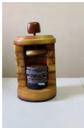
Figure 3. Third pile built: the apparatus is more similar to historical images, and it is able to light up a LED. A screw thread and a thin wood wall keep the plates as a pile. Source: the authors.
