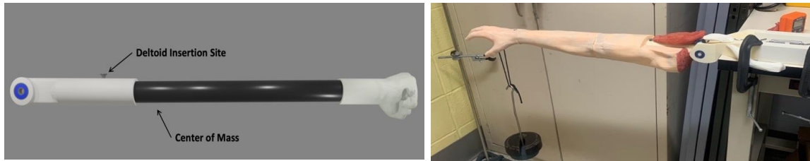
Figure 3. The first figure (left) shows the first arm model, and the second diagram (Right) shows the completed version of the 3D-printed arm. We used a metal rod to add weight to the arm.
