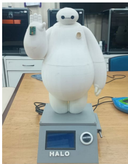
Figure 4. Final prototype in operation, demonstrating the simultaneous measurement of vital parameters and the display of data, integrated into a design focused on pediatric care.
